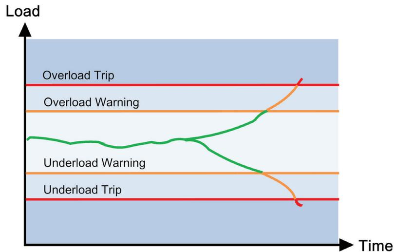
*Emotron M20 shaft power monitor protects your pump and process against damage and downtime. Early warnings and trips allow preventative action to be taken.*
