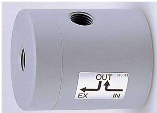
'Quick Exhaust Valve' prevents corrosion of the solenoid valve when adverse operating conditions arise. Installed between the pump and the solenoid valve, the QEV exhausts corrupt air or fluid before it can damage the solenoid.
